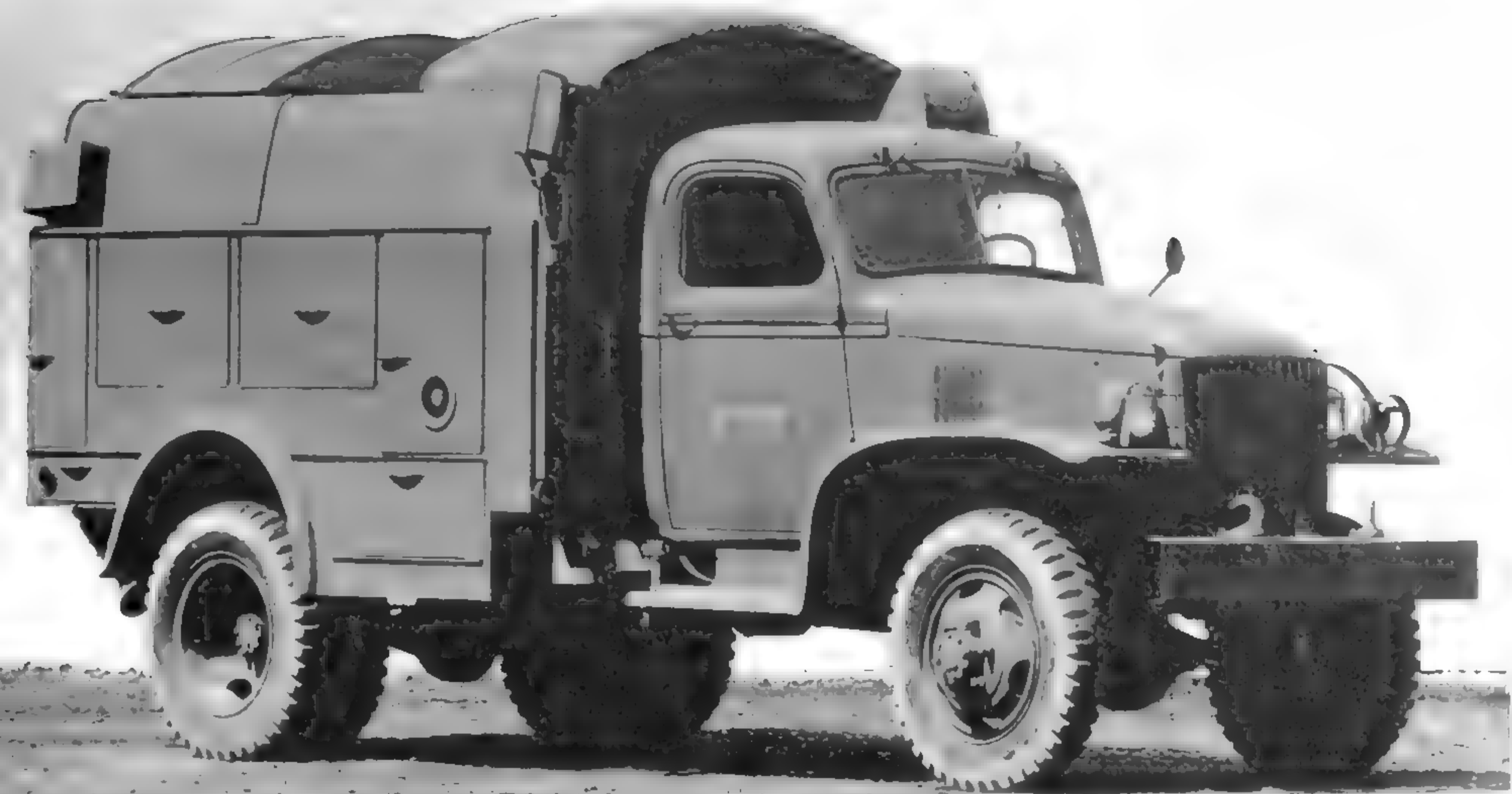
The G7173, also known by the Signal Corps nomenclature K43, was often used as a companion to the G7163. It was a telephone line maintenance truck. Several compartments were provided for tool and supply stowage, and the rear winch was also provided with extension shafts to drive an external cable reel. The shaft can be seen extending through the door of the first tool compartment behind the passenger. (U.S. Army photo)
